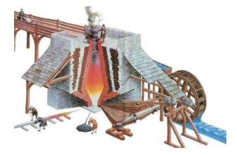
Above: An iron furnace powered by water. Notice the giant bellows adding oxygen to raise the heat in the furnace. The molten iron flowed out into sand forms that resembled suckling pigs. Hence the term pig iron.
